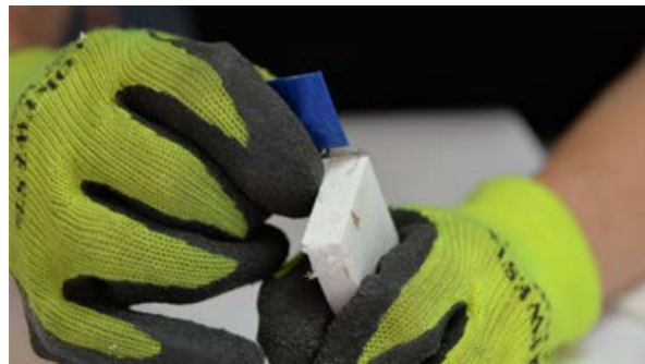
Using a stanley knife blade to finish off the rough edge
