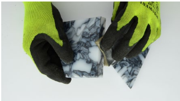
Use a scotch brite pad to remove light marking
