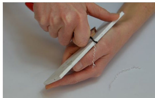
Starting from one corner pulling the deburring tool along the edge of the plastic just as shown above.
