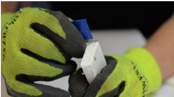
Using a stanley knife blade to finish off the rough edge
