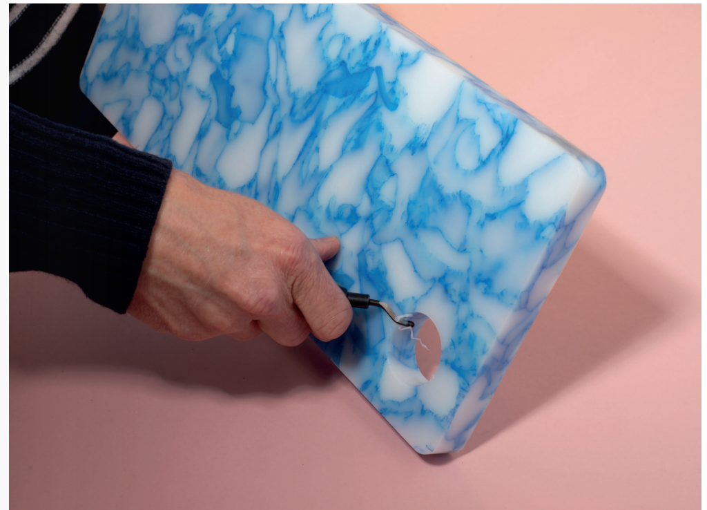
↑ Hand deburring to create a soft, rolled edge
