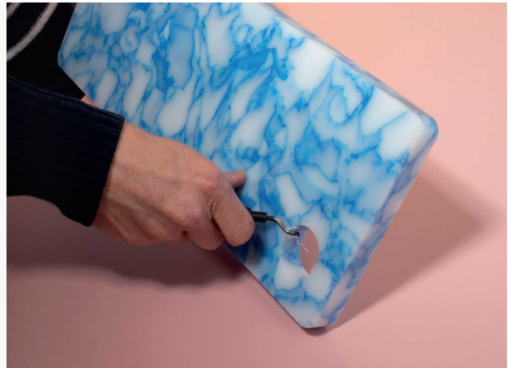
↑ Hand deburring to create a soft, rolled edge
