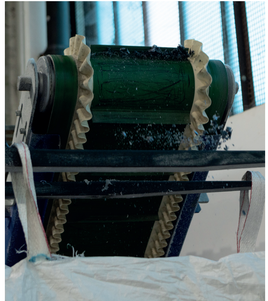
↑ In-house granulation of skeletal sheet waste
